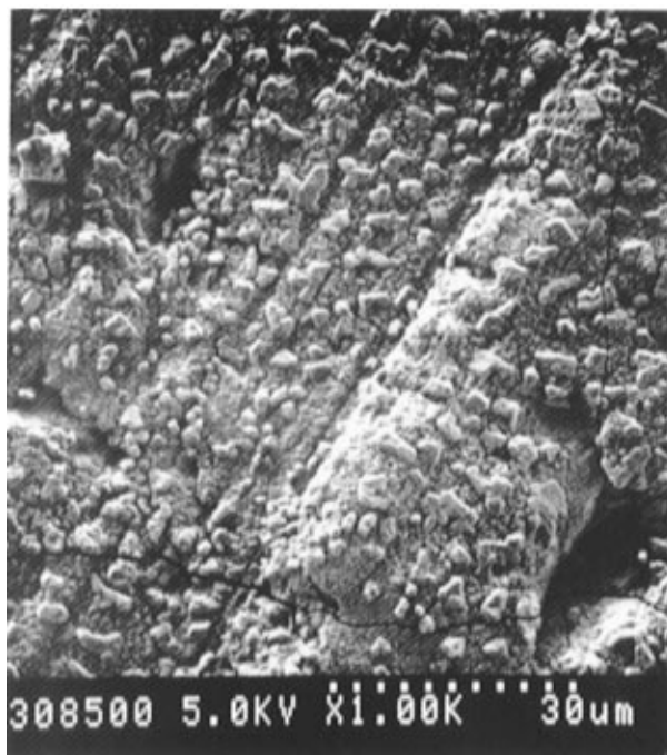
Figure 10. SEM micrograph of fused pellet after 2 h dissolution in a flow cell (flow rate 4 \times 10^{-2} \text{ cm}^3 \text{ s}^{-1} ). The dotted bar represents a distance of 30 \mu\text{m} .
